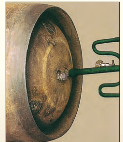
The tests conducted in the presence of DOT representative and repeated in California, confirmed that when over-pressurized, the chimed ends opened and the head reversed, providing additional volume and enhanced safety
