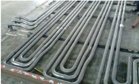
Super Heater Coils
