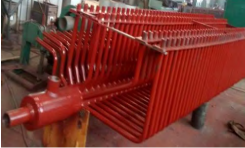
Primary Super Heater Header
