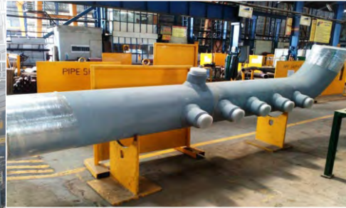
Pre-Fabricated Piping Spool
