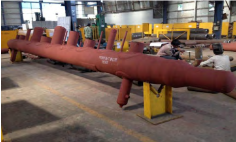
Main Stream Piping Spool
