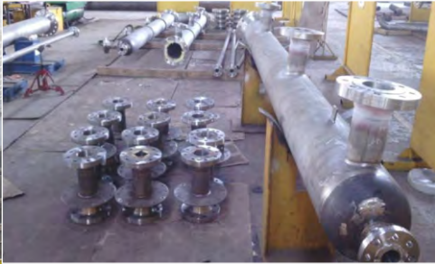
Compressor Piping Spools
