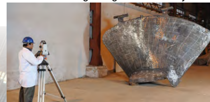
Profile measuring using Theodolite System
