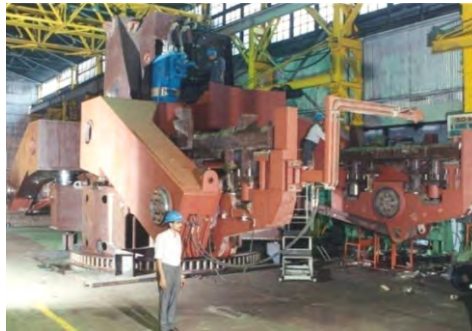
Ladles Turret for Steel Melting Shop (SMS)
