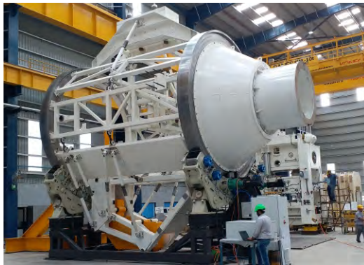
Gantry for Proton Beam Therapy Equipment (Cancer Research)
