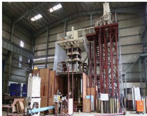
Nuclear Waste Compaction Press
