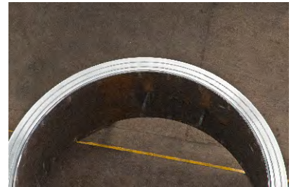
Shrink fitting of Multi-Wall type Vessels
